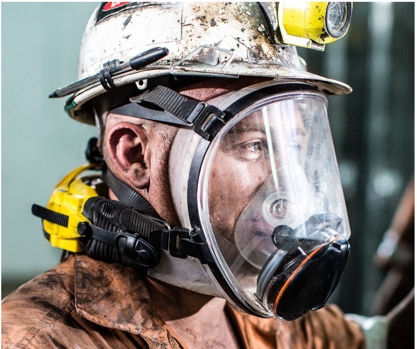
Fig 5. PAPR systems incorporate face and eye protection and need to be compatible with other PPE.
