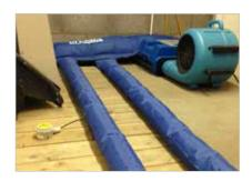
Octopus System This system is great to dry under timber floors that are on battens.
