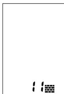
1. Once on the material menu press the "M" button to change the material (material #/type should start flashing).
