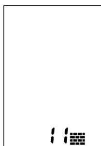
1. Once on the material menu press the "M" button to change the material (material #/type should start flashing).
