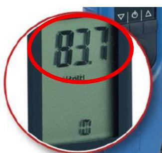
Compare the two readings. As the reading is relative, you can only gauge the increase of moisture to the affected area by the variance between the two numbers.
