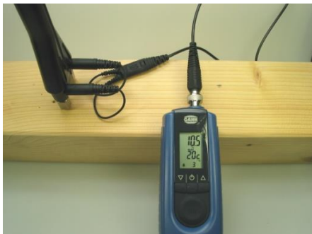
Figure 4-3 Measuring across the fibre direction with M 20
