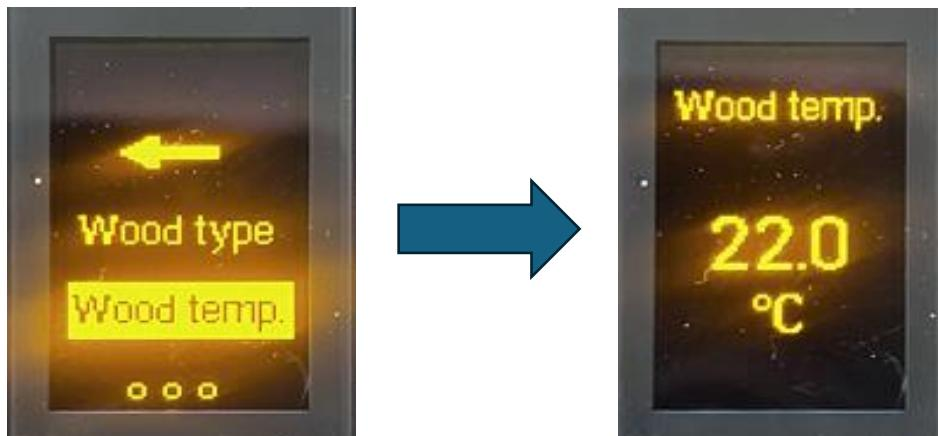
**Step 8:** Navigate back to the measuring menu by pressing "M" with the selected. Hold "M" with the electrodes in the material. Release "M" to save the reading.
