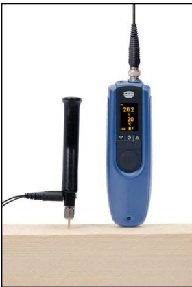
Figure 5-1: Measuring across the fibre direction with M 20
