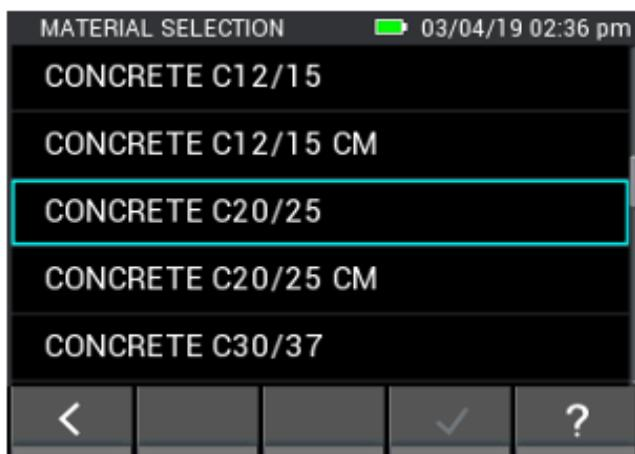
Scroll through the materials using touch screen until you are on the desired type.
