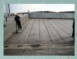
With MOIST SCAN there is a new instrument available for fast scanning of moisture distributions on large area flat roofs. By microwave scanning roof areas up to ten thousand square meters can be investigated very quickly. The lateral resolution achievable with the microwave scanner is in the order of 10 cm. For small areas it can be reduced down to 5 cm.
