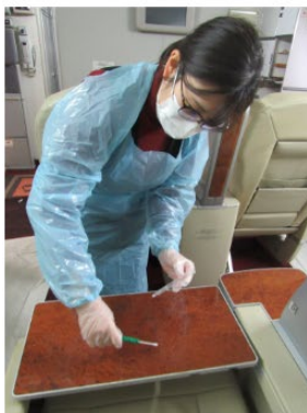
The Kikkoman A3 is used to quantify the cleanliness of various places that customers come into contact with. This is an evaluation of in-flight tables.
