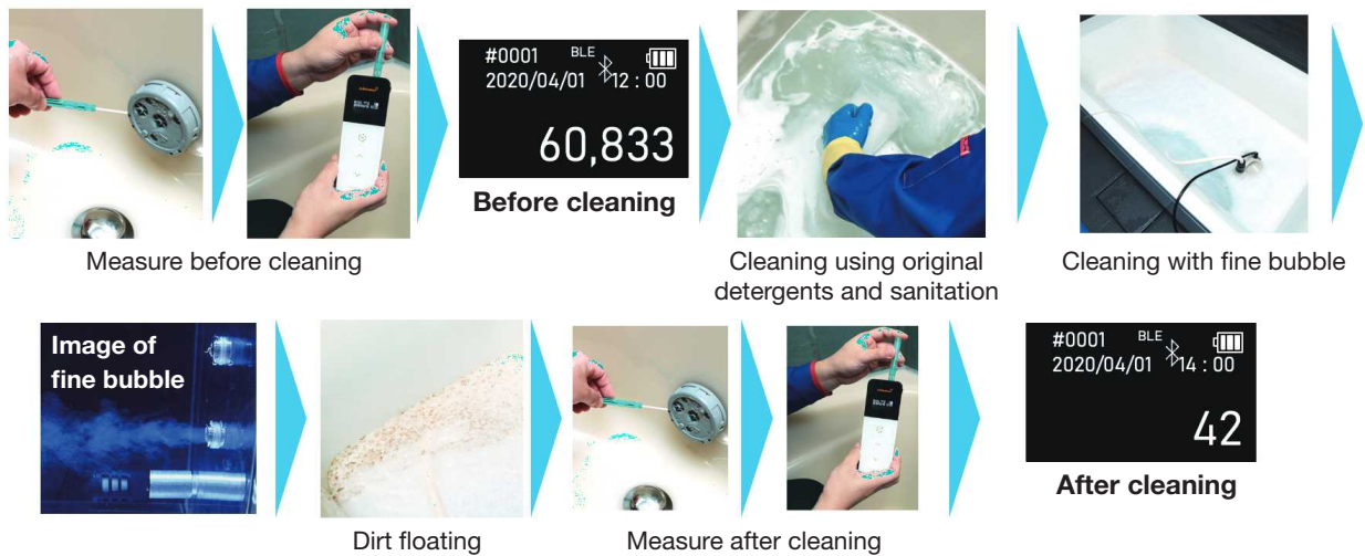
Photo 2 : Example of using ATP Test (Kikkoman A3) in the cleaning service business
