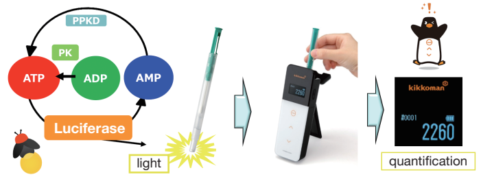
Figure 3 The principles of ATP Test (Kikkoman A3)
