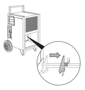
Check whether the hose is properly positioned on the connection. Screw it on to the device connection as illustrated.
