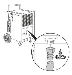
4. Guide the other hose end to a suitable drain or sufficiently dimensioned collection container. Please note that the hose must not be kinked.
